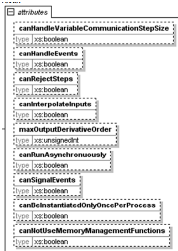
Figure 17: Capability flags of FMI for Co-Simulation
