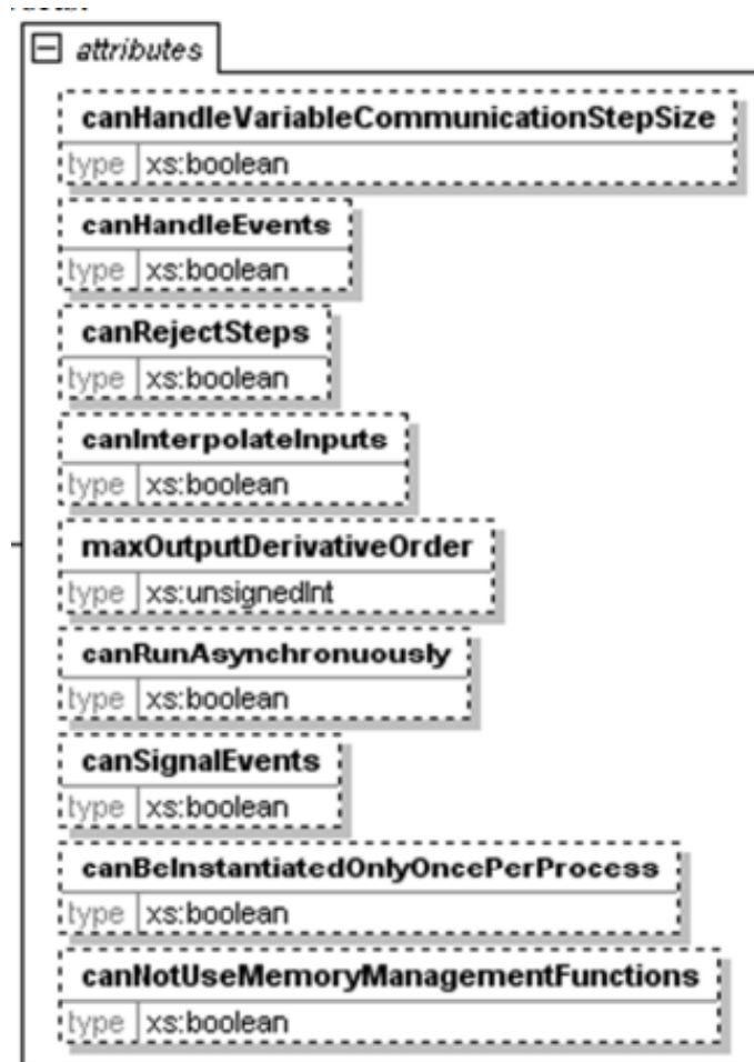
Figure 17: Capability flags of FMI for Co-Simulation
