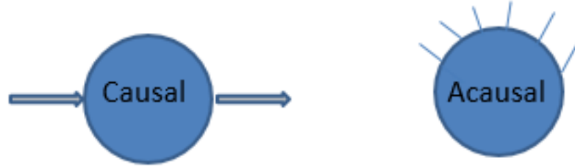
Figure 8: causal approach (oriented) / acausal approach (unoriented)
