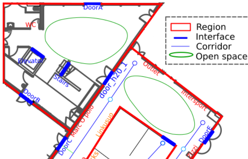
Figure 5.4: Representation of the semantic model of the environment used for route description.
