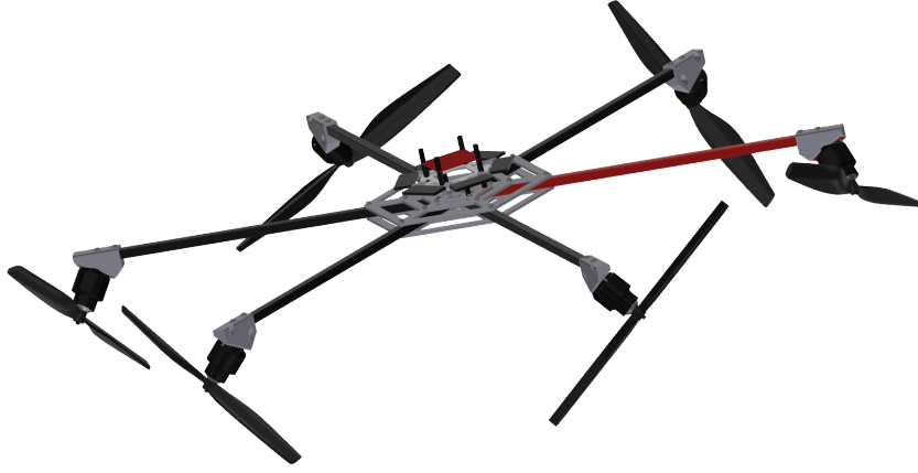
Figure 6.6 – CAD model of the Tilt-Hex prototype.
