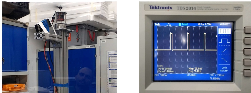
Figure 6.18 – Setup used for the identification of the propeller parameters. Left : actuator mounted on top of a force/torque sensor. Right : oscilloscope to measure the PWM pulse width of the commands. Relating these data allows to determine the propeller parameters.
