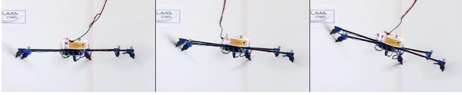
Figure 7.6 – The Tilt-Hex performing Exp. 1.1 at different time instances: left : t = 15.4 s; center : t = 37.7 s; right : t = 47.9 s. Although the reference orientation is constant and horizontal, the Tilt-Hex adapts it to allow the prioritized tracking of the reference position.
