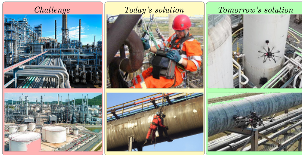
Figure 1.4 – An example of aerial physical interaction task: the inspection with contact of oil/gas pipelines. Left : the addressed scenario. Center : the solution today, achieved by human operators. Right : the solution tomorrow in the vision of the AeroArms project, with the task performed by aerial robots.
