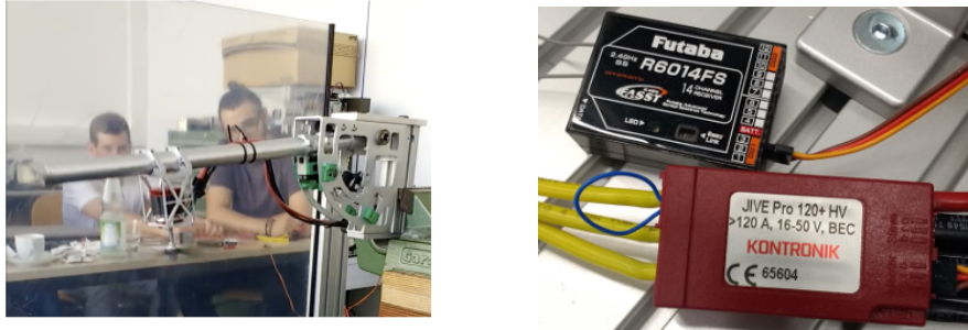
Figure 6.17 – Left : leg lifting test in the worst operational mode (spinning in the 'opposite' sense). Right : ESC and receiver used for the identification of the propeller parameters.
