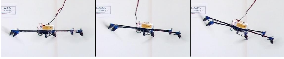
Figure 7.6 – The Tilt-Hex performing Exp. 1.1 at different time instances: left : t = 15.4 s; center : t = 37.7 s; right : t = 47.9 s. Although the reference orientation is constant and horizontal, the Tilt-Hex adapts it to allow the prioritized tracking of the reference position.
