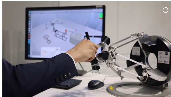
Figure 11.1 – Photo of a human operator controlling the state of the simulated Tele-MAGMaS system with an Omega.6 haptic device.
