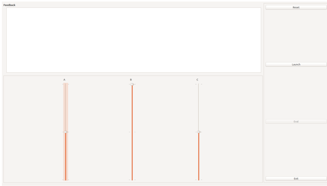
Figure 4.1: Screen shot of the interface used by the participants to set the kinematic bounds. A was for acceleration, B for jerk, C for speed. Participants didn't had this information. We can also see a launch button used to begin a new test, and an eval button that opens a new Godspeed questionnaire to fill.
