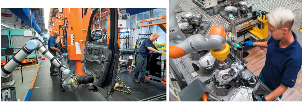
(a) A universal cobot used in car assembly production line. (b) LBR iiwa of KUKA cooperating with BMW employee in Dingolfing's factory.
