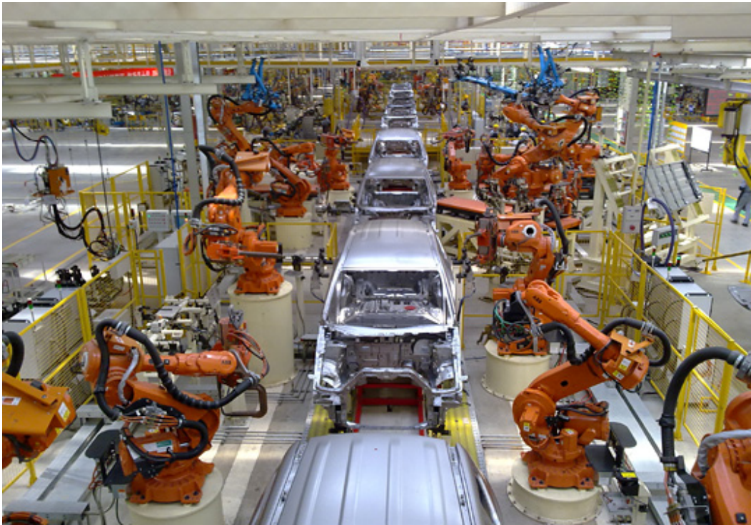
Figure 1.4: A typical assembly line composed of robotic arms confined in cages.
