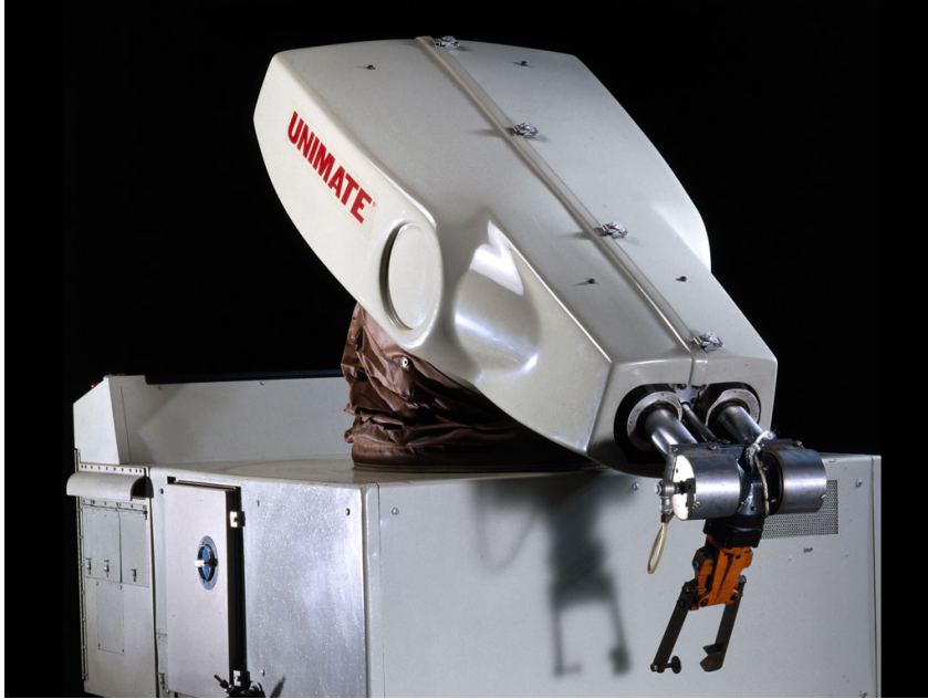
Figure 1: Unimate, the grandfather of industrial robots.
