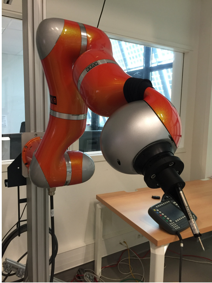
Figure 3.12: A KUKA LWR4 robotic arm used for our experiments.
