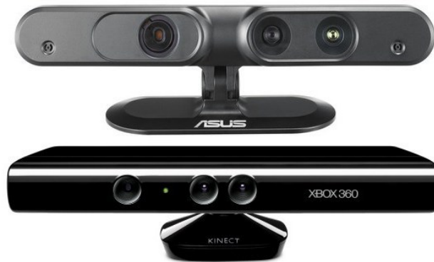
(b) Kinect XBOX360 and Asus Xtion. These cameras are mainly used for QR code tracking.
