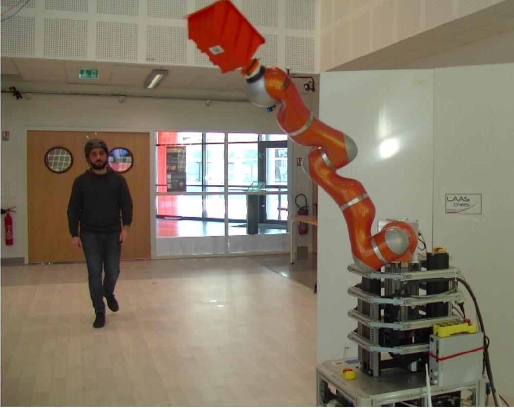
Figure 3.18: Experiment illustration (see [video-1]). The robot is accomplishing a task while a human is walking towards it. The trajectory planner is informed by the motion capture system (helmet) of the human presence and adapts its behaviour accordingly.
