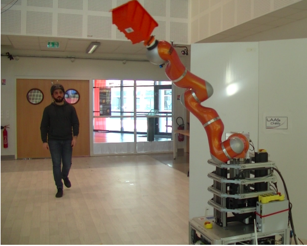
Figure 3.18: Experiment illustration (see [video-1]). The robot is accomplishing a task while a human is walking towards it. The trajectory planner is informed by the motion capture system (helmet) of the human presence and adapts its behaviour accordingly.
