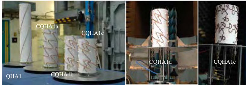
Figure 3. Manufactured wire-supported CQHAs derived from QHA1 using as shaping function various combinations of sine functions (CQHA1a, CQHA1b, CQHA1c and CQHA1d) and prefractal (Von Koch) profile combined with a sine function (CQHA1e).
