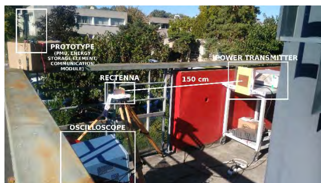
FIGURE 13. Photograph of our experimental outdoor setup (SN powered by using a WPT technique).
