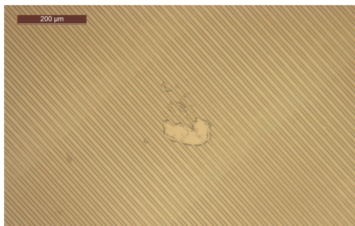
Figure 3.36.: Optical microscope observation of the center of the coverslip, 10x magnification. The sample was exposed with a dose of 50 \text{ mJ.cm}^{-2} . Resist motifs appeared wide and under-developed.
