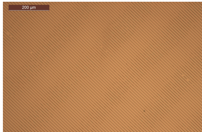
Figure 3.39.: Optical microscope observation of the center of the coverslip, 10x magnification. The sample was exposed with a dose of 100 \text{ mJ.cm}^{-2} and developed for 60 seconds in CD MF-26. Resist motifs appeared well-defined and continuous.
