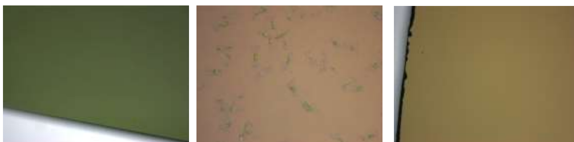
Figure 3.7: Optical microscopy images of the surface of a [\text{Fe}(\text{HB}(\text{tz})_3)_2] film before (left) and after (middle) the deposition of a layer of SiOx by PECVD. A witness surface (substrate only) is also shown after PECVD deposition (right).
