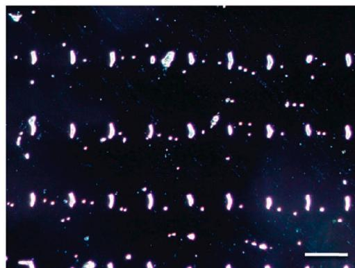
**Figure 6.** Patterned bacteria onto functionalized surface with 3-aminopropyltriethoxysilane (APTES) ( $1100 \times 1000 \mu\text{m}^2$  dark field image with a scale bar that measures  $30 \mu\text{m}$ ). Reproduced with permission from [55].
