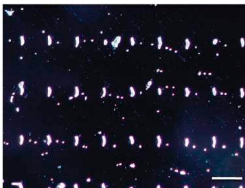
Figure 6. Patterned bacteria onto functionalized surface with 3-aminopropyltriethoxysilane (APTES) ( 1100 \times 1000 \mu\text{m}^2 dark field image with a scale bar that measures 30 \mu\text{m} ). Reproduced with permission from [55].
