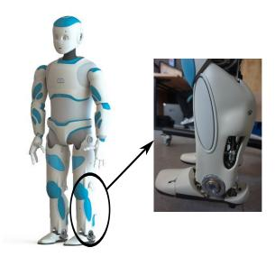
Figure 2.1: The leg of the robot Romeo is designed based on a screw-nut-cable actuator, which is shock-proof and low-friction, but induces flexibility due to the cable.
