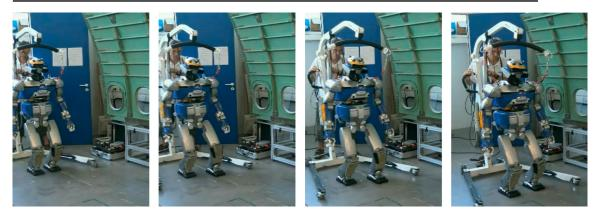
Figure 4.14: The experiment of walking forward when using the WPG with Laguerre basis functions.
