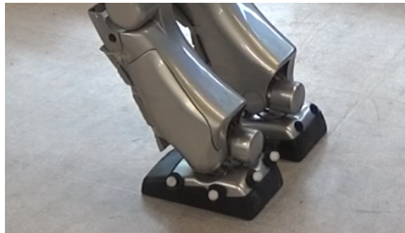
Figure 3.7: Reflectors on the left of HRP-2 form the pattern to be detected by motion capture
