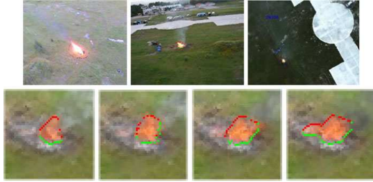
Figure 2.4: Aerial view of a wildfire from different angles ( top ). Algorithms are able to locate the position of the fire if a digital elevation map is provided ( bottom ). Excerpt from [Merino 2012]
