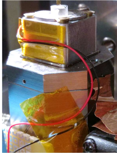
Figure 94: Picture of our scanning apparatus. One can recognize the high-BW Z-actuator block at the top with its electrical connections. On the bottom is the commercial scanner E-363 PicoCube.
