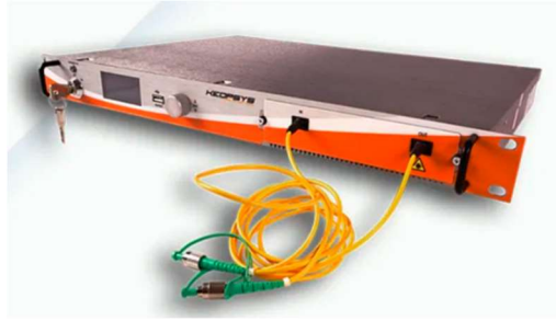
Figure C-7: Picture of the fiber amplifier used.
