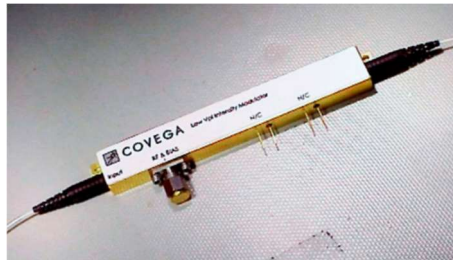
Figure C-3: Picture of an EOM. One can observe its input and output optical fibers on the left and right hand side of the picture. RF port, DC bias and photodiode pins can be seen on its edge. As a note, its integrated photodiode was sensitive to polarization so we did not use it to monitor power output.
