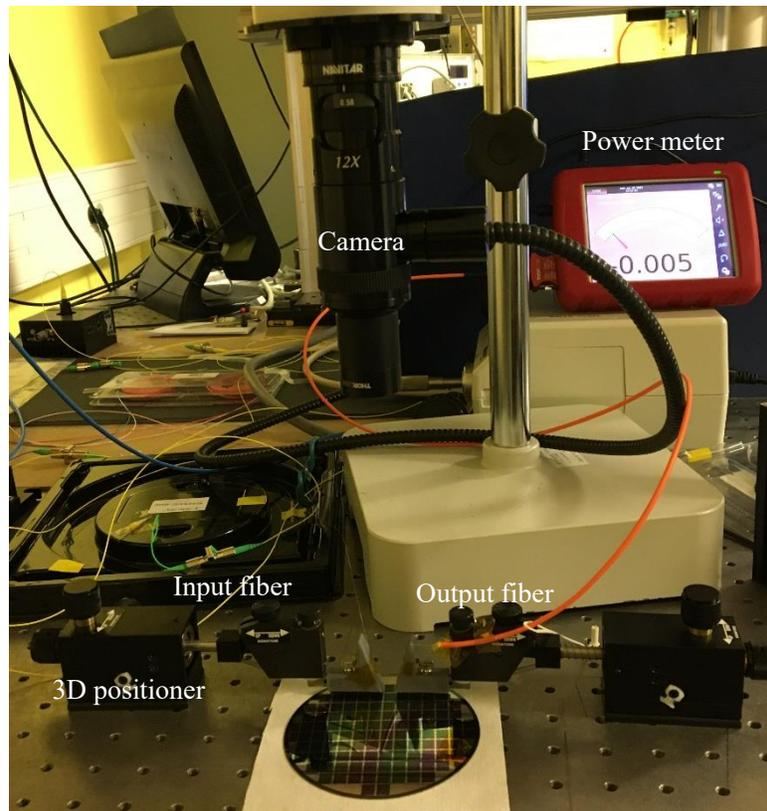
**Figure 103.** Improved optical bench for characterization of components.
