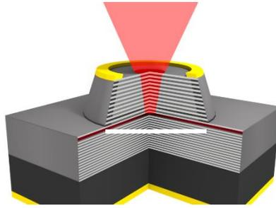
**Figure 15.** Schematic view of a typical GaAs vertical cavity surface emitting laser (VCSEL) with a short cavity length ( $\sim 1\mu\text{m}$ ) and a small, buried oxide aperture ( $\sim 4\mu\text{m}$ ) respectively leading to longitudinal and transverse single mode confinement and single mode operation.
