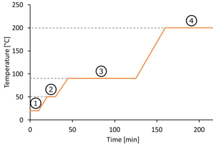
**Figure 69.** Gradually baking process of CYTOP polymer.
