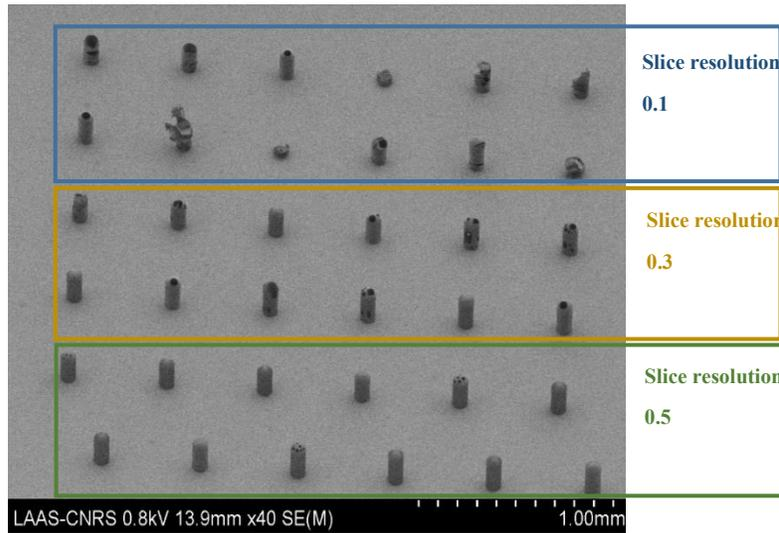
**Figure 42.** Calibration of exposure parameters for Nanoscribe writing.
