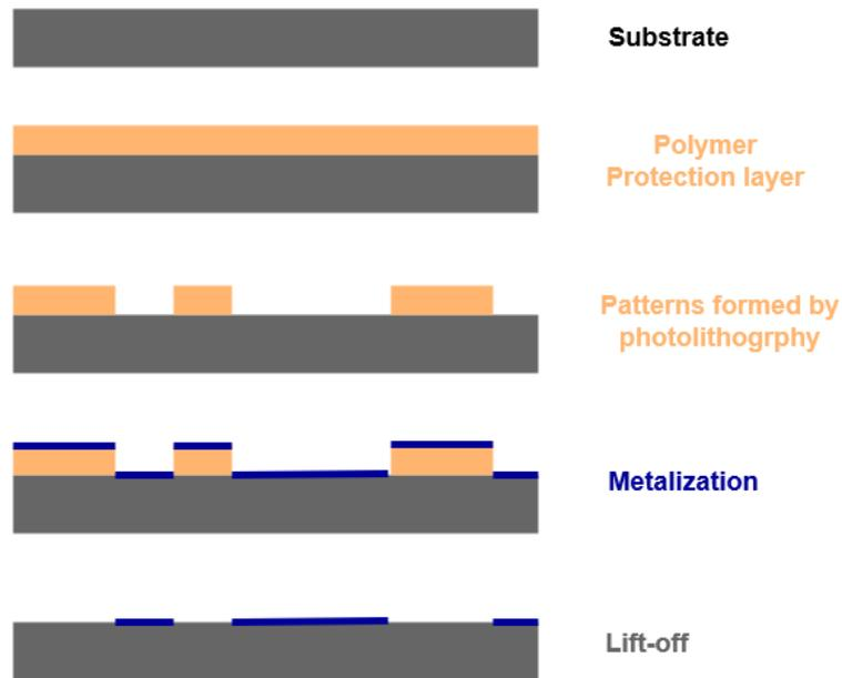
**Figure 75.** The manufacturing process flow of lift-off method.
