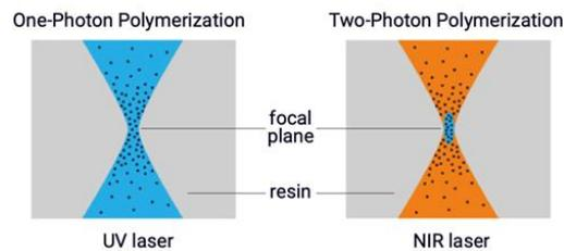
**Figure 38.** Comparison of one-photon polymerization and two-photon polymerization.
