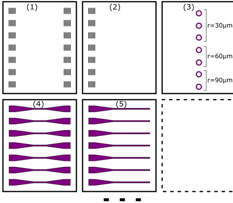
**Figure 65.** Schematic representation of the five over nine areas available on the reticle. Each pattern will cover a  $6.2 \times 7.2 \text{ mm}^2$  on the wafer. A complete micro-resonator will be a combination of three areas of the reticle. Note: the polarity is not respected for better graphic rendering of the schematic.
