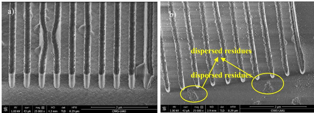
**Figure 99.** a) Protrusions appear next to grating coupler lines and pull the patterns to be distorted. b) A re-added plasma O<sub>2</sub> disperse the residues and contaminates the surface of sample.
