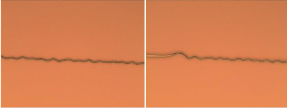
**Figure 85.** Distortions and misalignments of SU-8 waveguides on CYTOP lower cladding.
