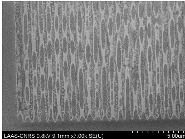
**Figure 74.** Aluminum grating coupler after Plasma etching.
