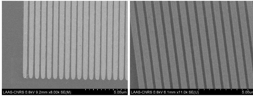
**Figure 78.** Aluminium grating couplers fabricated by lift-off process.
