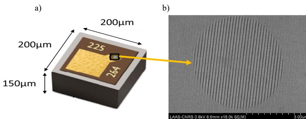
**Figure 19.** Single 850nm VCSEL chip with shallow etched grating at its surface (Trumpf).
