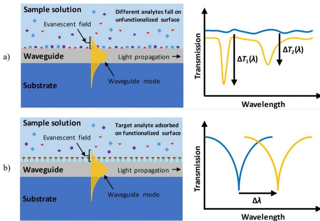
Figure 4. Two detection modes of microresonator sensors. [28]
