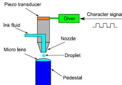
**Figure 27.** Schematic diagram of the inkjet printing setup [83]
