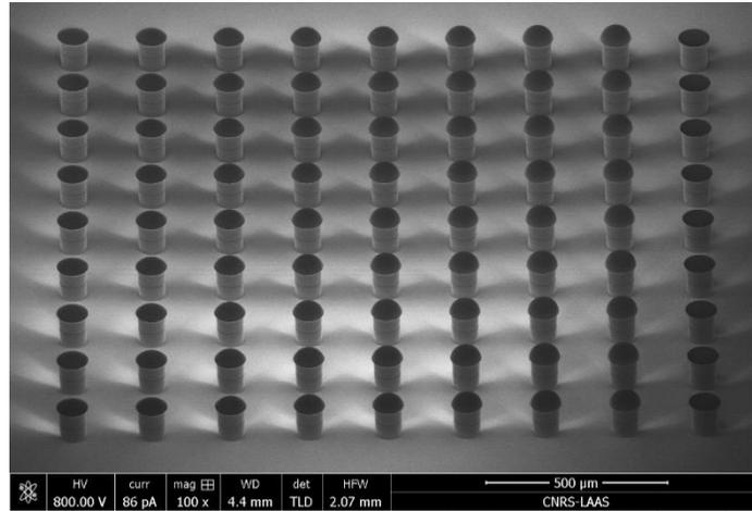
**Figure 28.** Pedestals array for calibration of lens thickness.
