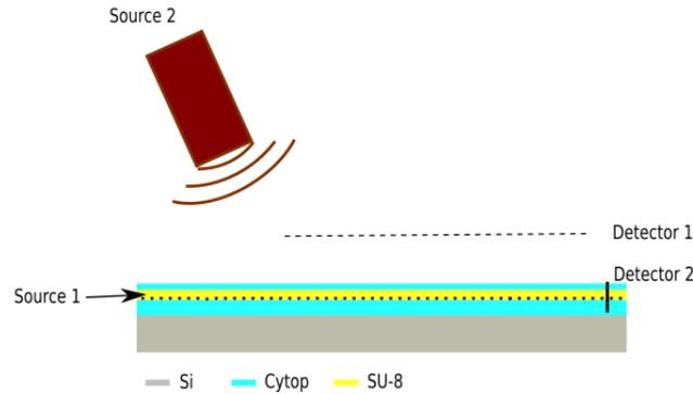
**Figure 55.** Schematic of the model simulated with Lumerical, showing the two input sources, and the position of the two detectors used in the simulation to optimize both output (Source 1 + Detector 1) and input (Source 2 + Detector 2) grating couplers.
