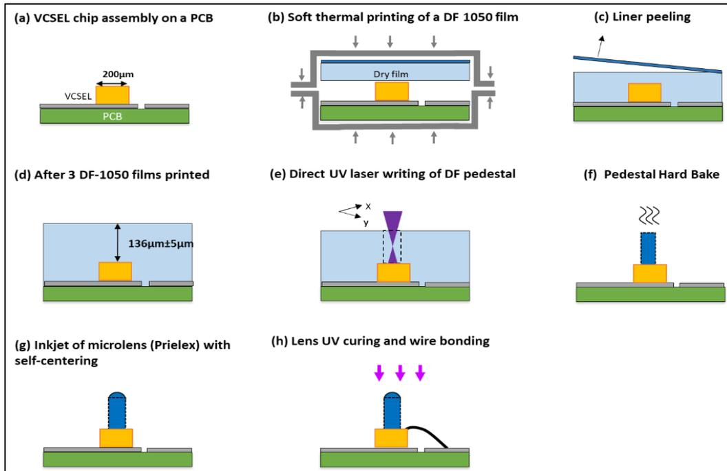
**Figure 24.** Procedure of VCSEL based micro-optical system fabrication. [82]
