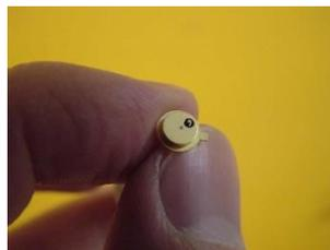
**Figure 7.** Image of a VCSEL chip mounted on a TO-46 header.
