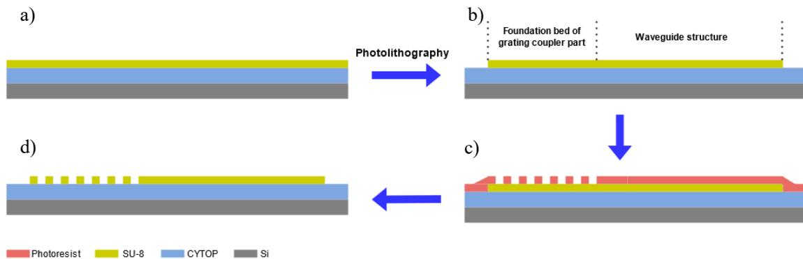
**Figure 9.** Schematic diagram of manufacturing process of SU-8 grating coupler by using stepper.
