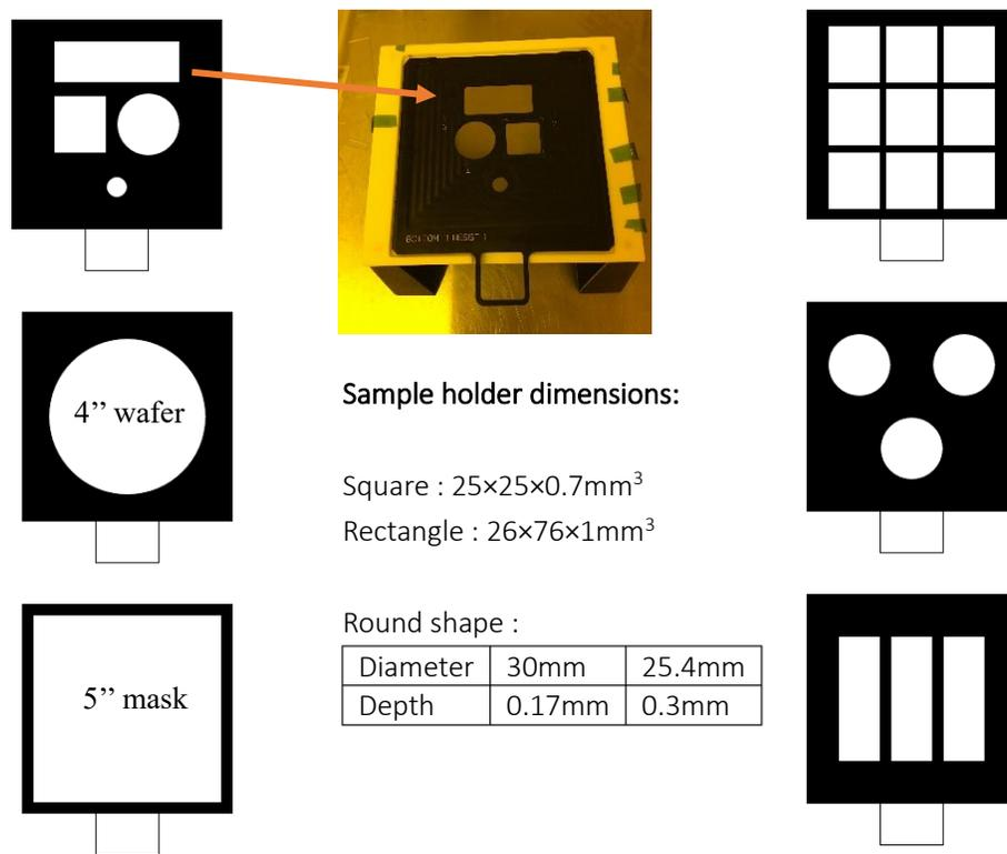
**Figure 40.** Different sample holders provided by Nanoscribe.
