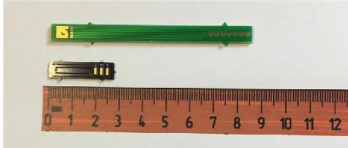
**Figure 20.** Illustration of the two kinds of PCB used in this study: the previous version on the top (green PCB) with a conventional thickness of 1.57 mm, and an optimized, thinner version at the bottom (purple PCB) with a lower thickness of 0.8 mm to fit the constraints of the Nanoscribe tray.
