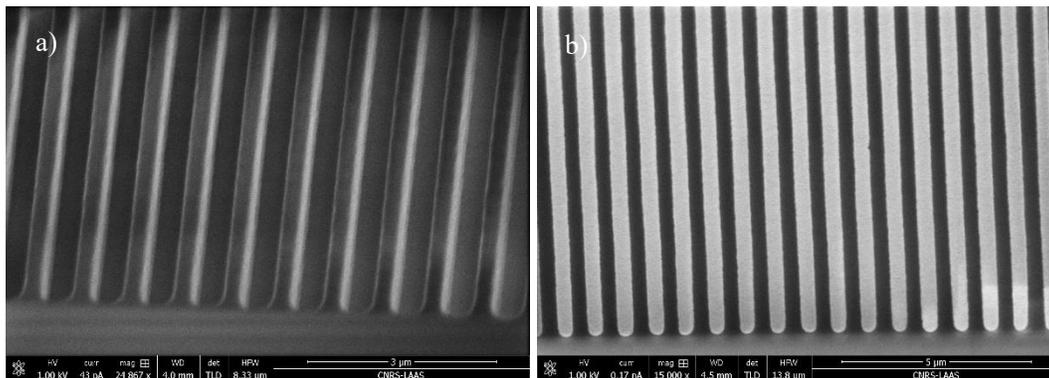
**Figure 84.** a) Grating coupler patterns in LOR+ECl obtained after photolithography with exposure doses between 1000 to 1100 J/m<sup>2</sup>. b) Aluminium grating coupler obtained after completion of the lift-off process.
