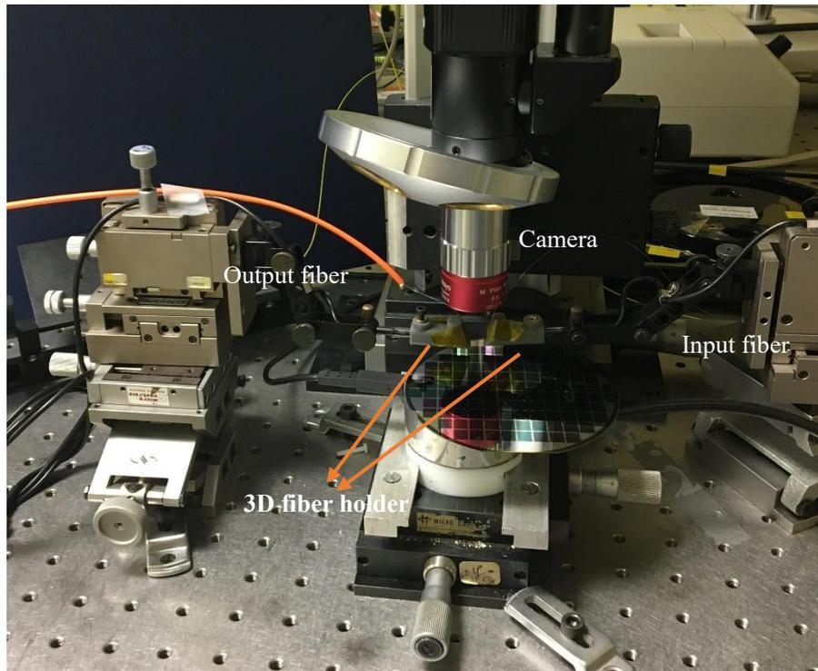
**Figure 104.** Upgraded optical bench for characterization of components.
