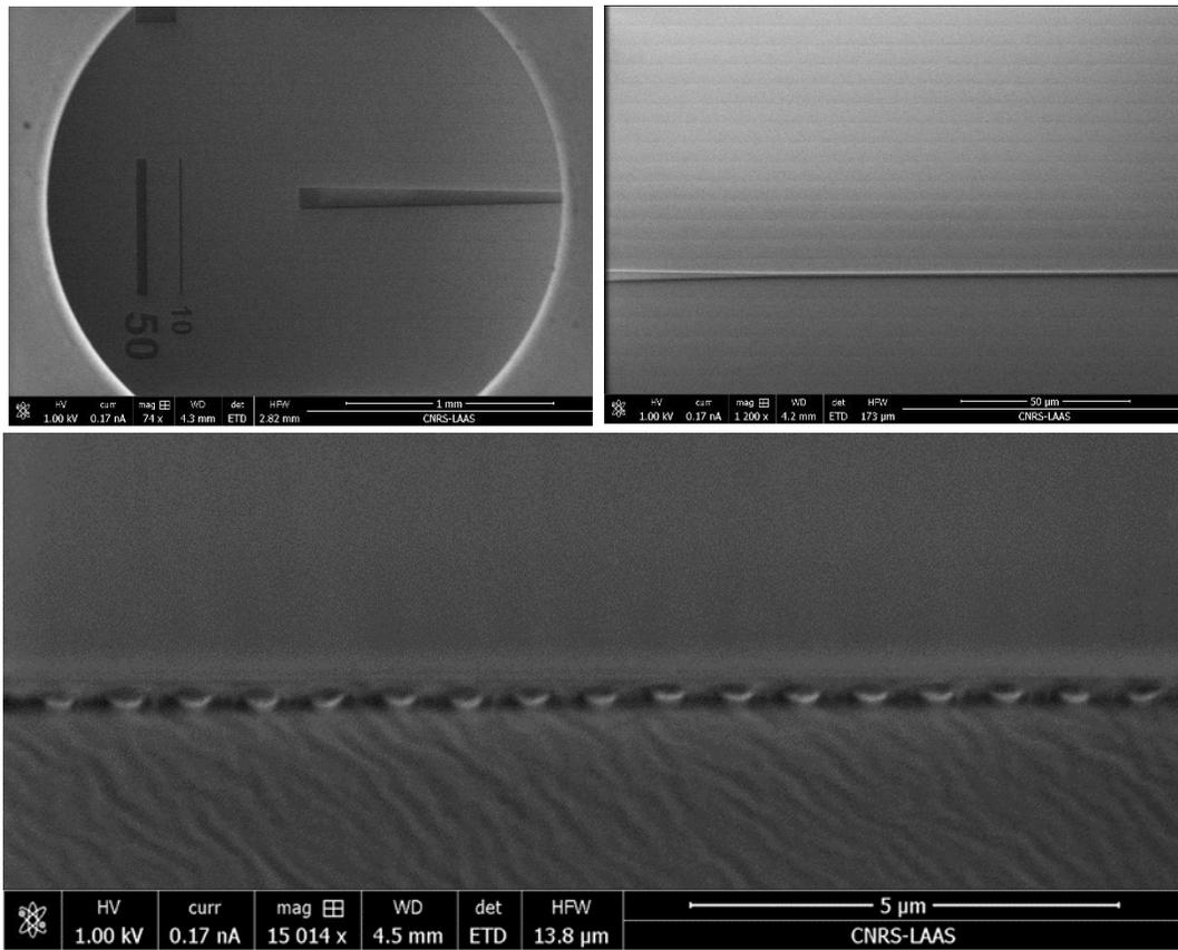
**Figure 86.** Upper left: SEM wide view of the tapered waveguide and the grating coupler realized over a CYTOP cladding. Upper right: Close-up view of the waveguide at its thinnest section (1 μm width). Bottom: Tilted SEM image at the edge of the taper, highlighting the smoothness of the surface despite the presence of the Al grating coupler.
