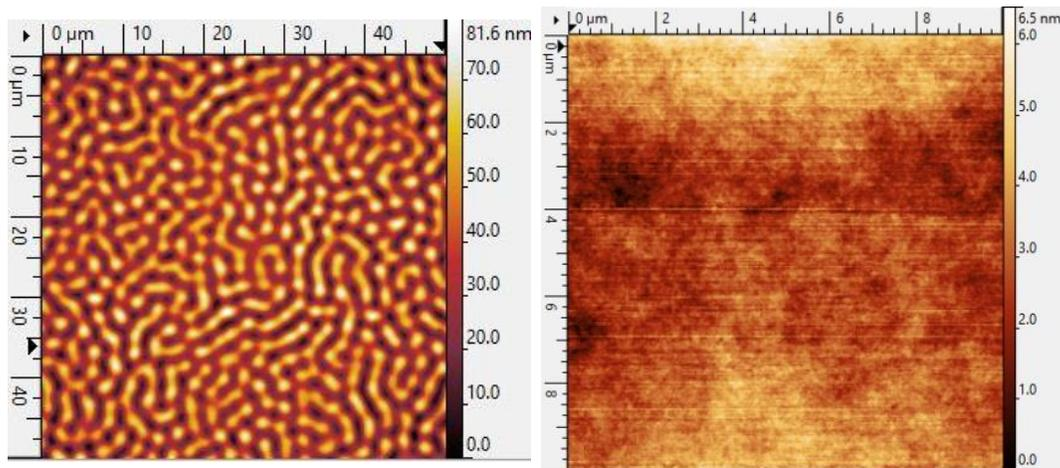
**Figure 89.** CYTOP surface before/after plasma oxygen etching.
