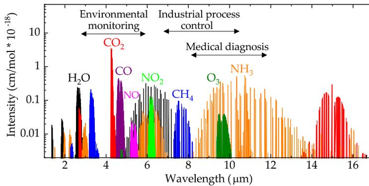
**Figure 3.** Absorption spectra of common gas molecules. [11]
