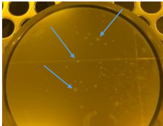
Figure 72. Bubbles that appear at the Al-CYTOP interface due to heating.
