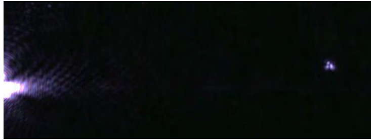
Figure 92. Incident light on the input grating (left) and output light obtained on the output grating (right) with an SU-8 waveguide covered on CYTOP lower cladding.
