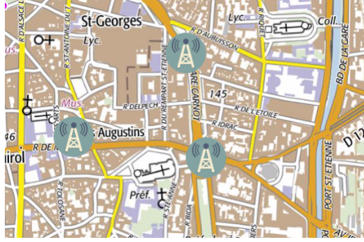
Figure 3.1: A selected area of Toulouse which is covered by three BSs (LTE1800) of the French mobile network operator Free Mobile.
