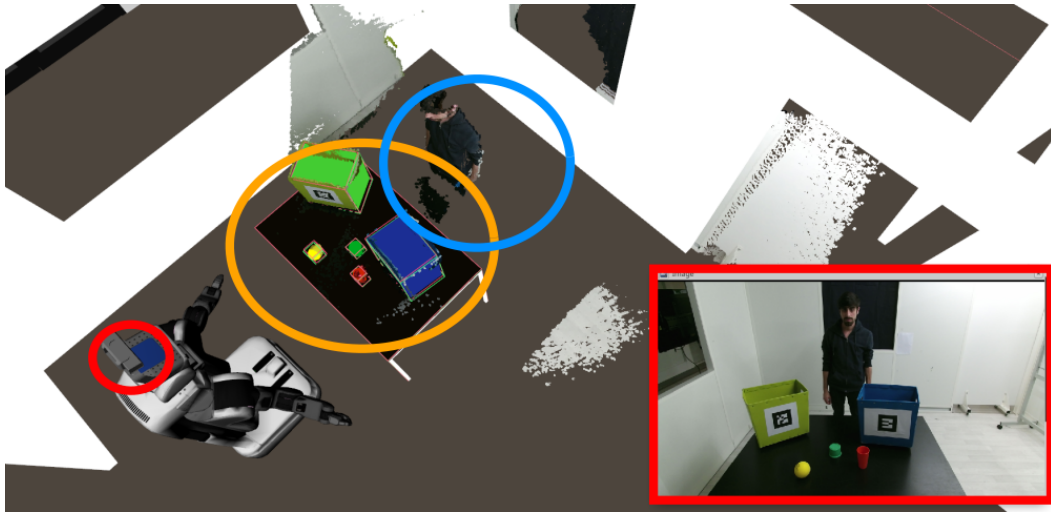
Figure 5.2: The red circle indicates where the Kinect2 RGBD sensor is positioned, and the red rectangle indicates the camera view of the sensor. The orange circle indicates where interaction takes place, and the blue circle where the human is placed.
