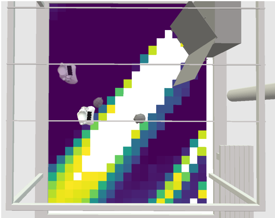
Figure 4.4: Costmap computed by the pointing planner, which allows computing the desired position for the human and the robot. In blue are the area where the landmark is visible, In yellow is the area where the landmark is barely seen, and in white where it is not visible.
