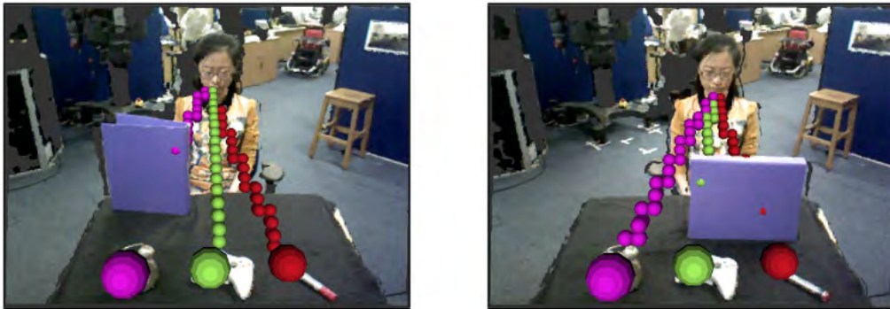
Figure 2.4: Level 1 perspective taking with voxel based representation adapted from [Fischer 2016]. Here a discrete raycasting approach in the voxel based representation is used to compute the visibility of objects.
