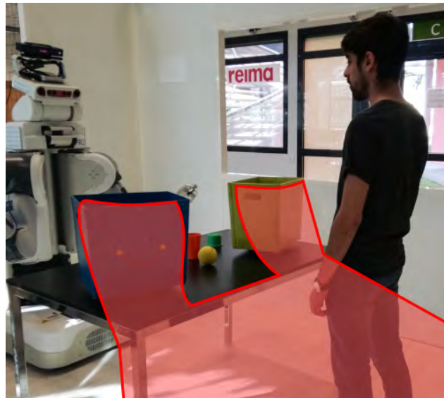
Figure 5.1: Our experimental setup setup with a PR2 robot. From the point of view of the robot, a part of the scene is occluded (colored in red in the picture).
