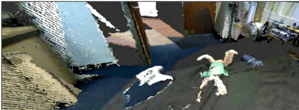
Figure 2.5: Level 2 perspective taking with point-cloud based representation adapted from [Fischer 2016]. Here a rotation of the point cloud is used to reconstruct the image from the human point of view (assuming that the environment is already known).
