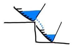
Figure 1.2: The water clocks were based on flows. The problem with the earliest versions was that the flow was irregular (the lower is the water level in the first container, the slower the water flowed into the second container).
