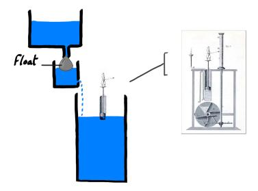
Figure 1.3: Ctesibius' solution for controlling the diminishing flow consisted in adding a third container between the two existing containers. Using a float regulator system, the Ctesibius' water clock required no outside intervention between the feedback and the controls of the mechanism.
