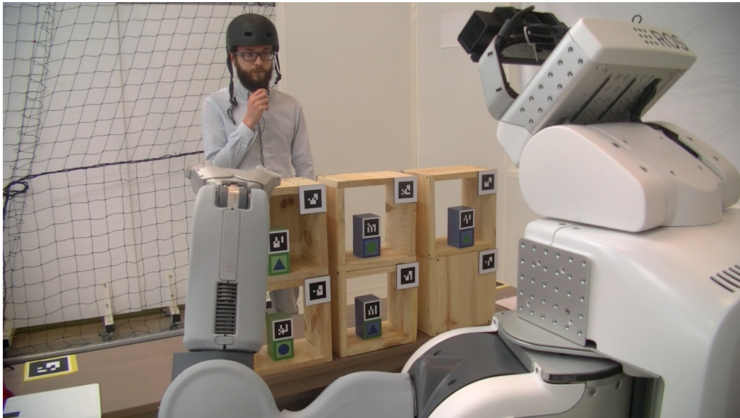
Figure 9.7: Initial configuration for both case studies. The top-right block is not visible, and thus unknown, by the human partner. The robot can not know if there is a block in the bottom-left compartment. All other blocks are known by both the robot and the human.
