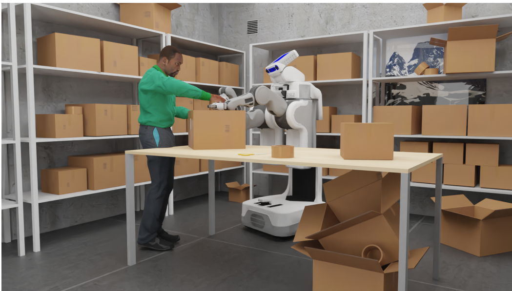
Figure 1.2: A PR2 robot and a human employee collaborating to close a box.
