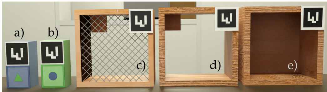
Figure 9.2: Part of the material used for the Director Task. Each element is equipped with AR-tags allowing their detection by the robot. Each block has four visual characteristics: a main color, a border color, a geometric figure and a figure color.
