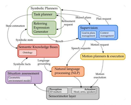
Figure 5.10: The architecture used to validate the method. The knowledge bases are continuously kept up to date through the situation assessment. The task planner can query the REG to estimate the feasibility and cost of future communications.
