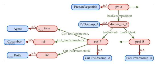
Figure 6.7: A graphical representation of the instance of a decomposition of the abstract task *PrepareVegetable*.
