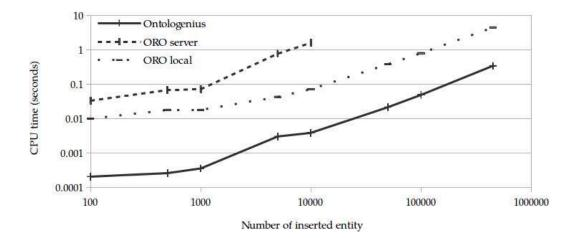
Figure 2.13: Comparison of the required CPU time for querying all the entities being animals, after that N entities have been created. Ontologenius and ORO are used with their own communication layer. To assess the impact of the communication layer on ORO performance, we also provide measures without the ORO communication layer (ORO local).
