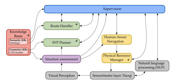
Figure 8.2: The general architecture developed for the robot guide. The components presented in this chapter are the colored blocks. The red components with the symbol \* are the ones on which I participate. The visual perception and dialogue components have been respectively developed by IDIAP and HWU and are described by [Foster 2019]. Naoqi is a Softbank Robotics software.
