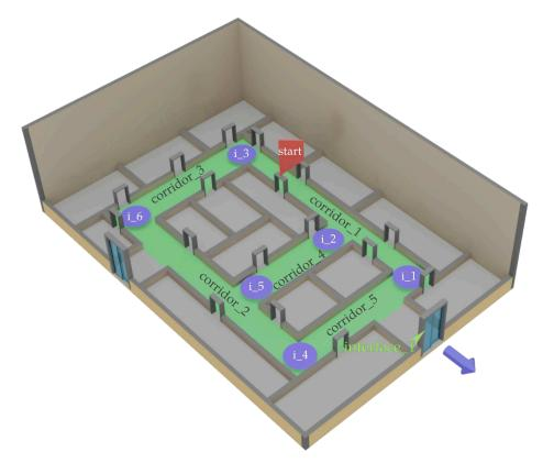
Figure 3.7: Representation of *region\_1* at the place-level. A region is composed of paths (here corridors only) connected through intersections. We know that the starting point of the search is along *corridor\_1* and the local goal place is in *corridor\_5*.
