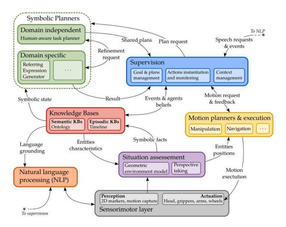
Figure 9.5: An overview of the cognitive architecture developed to handle the Director Task. Each block does not necessarily represent one software component but rather an architectural module (in terms of the features it implements). The arrows represent the type of information exchanged between the modules. This architecture extends the ones presented all along with this thesis.
