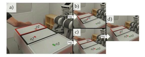
Figure 5.1: A Human-Robot collaborative task with three colored areas and three RFID tags (situation a). The robot has to explain to its human partner to put the tag o1 in the black area and the tag o2 in the white area, to reach the situation d. The objects identifiers' are only known to the robot. If all the communications of the task are not planned ahead, a deadlocked situation could appear if the robot first asks to move the tag o1 before o2 (situation b).
