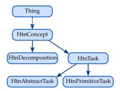
Figure 6.5: The upper classes used to decribe an HTN.
