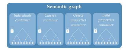
Figure 2.6: The semantic graph has four containers, one for each type existing in an ontology (i.e individuals, classes, object properties, and data properties). The containers own the nodes representing the elements of the ontology and store them in maps where the keys are the identifiers of the elements and the values are the nodes themselves. Each container also provides a lock mechanism allowing to prevent concurrency issues in multi-thread usage.
