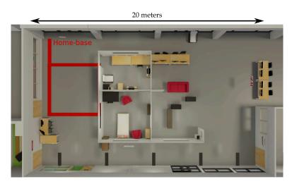
Figure 8.3: The 3D mesh model of the mockup mall at laboratory. The red square represent the interaction area as a square of 4 meters per 4 meters. Signs representing the shops have been place all around the environment.
