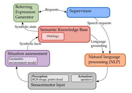
Figure 4.11: The architecture used to validate the method. The knowledge base is continuously kept up to date through the situation assessment.
