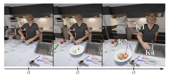
Figure 6.1: Referring to knife k2 in the current situation (t3) is impossible if the robot is performing an action that does not allow it to see what is in front of the human. Considering previous steps of the human's task, the robot can refer to the knife through the action to cut a tomato (t2) or to cut a cucumber (t1).
