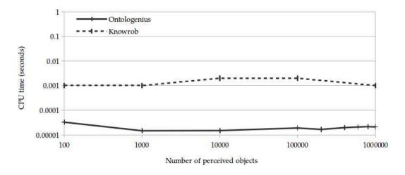
Figure 2.12: Comparison of the required CPU time for querying the pose matrix of a randomly selected object after that N perception entities have been created. Ontologenius is used without the ROS communication layer to provide comparable usage and thus results.
