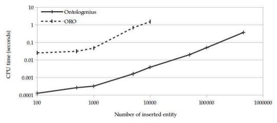
Figure 2.14: Comparison of the required CPU time for querying all the entities having a relation of the kind "isUnder" toward a given entity. Since the invert relation has been inserted for all the created entities, the software has to solve the inverse relation to answer the query. Ontologenius and ORO are used with their own communication layer.
