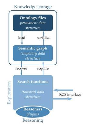
Figure 2.4: The software architecture of Ontologenius to manage a single Knowledge Base in the form of an ontology.
