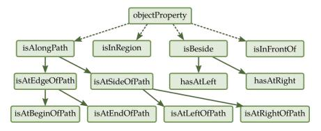
Figure 3.3: Representation fo the RBox (properties hierarchy) of the Semantic Spatial Representation used to describe the topology of an indoor environment.
