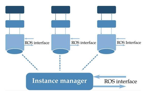
Figure 2.7: The software architecture of Ontologenius to manage multiple Knowledge Bases in the form of an ontology. An instance manager makes the link between each instance (see Figure 2.4) and has a direct access to each semantic graph to propose queries.
