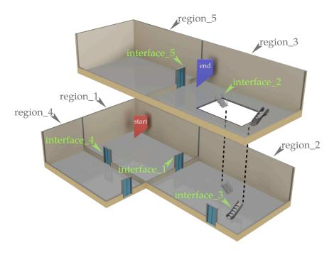
Figure 3.5: Representation of an environment at the region-level. Regions are linked through interfaces. We know that the starting point of the search is in *region\_1* and the goal place is in *region\_3*.
