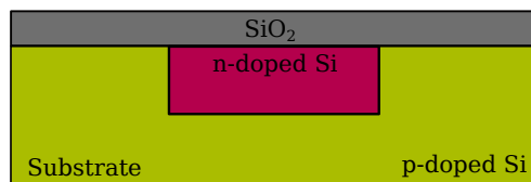
Figure 1.7: Cross-section view of a CMOS photodiode.
