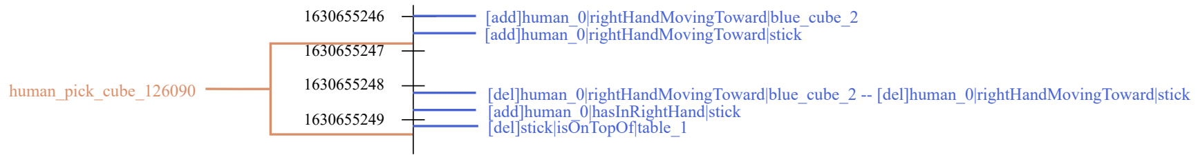
Figure 6.14 – Timeline produced by Mementar on which appear facts from perception (blue, on the right) and the action added by the Human Plan Manager based on data from the Human Actions Recognition (orange, on the left). Numbers on the axis are time in milliseconds (epoch time).
