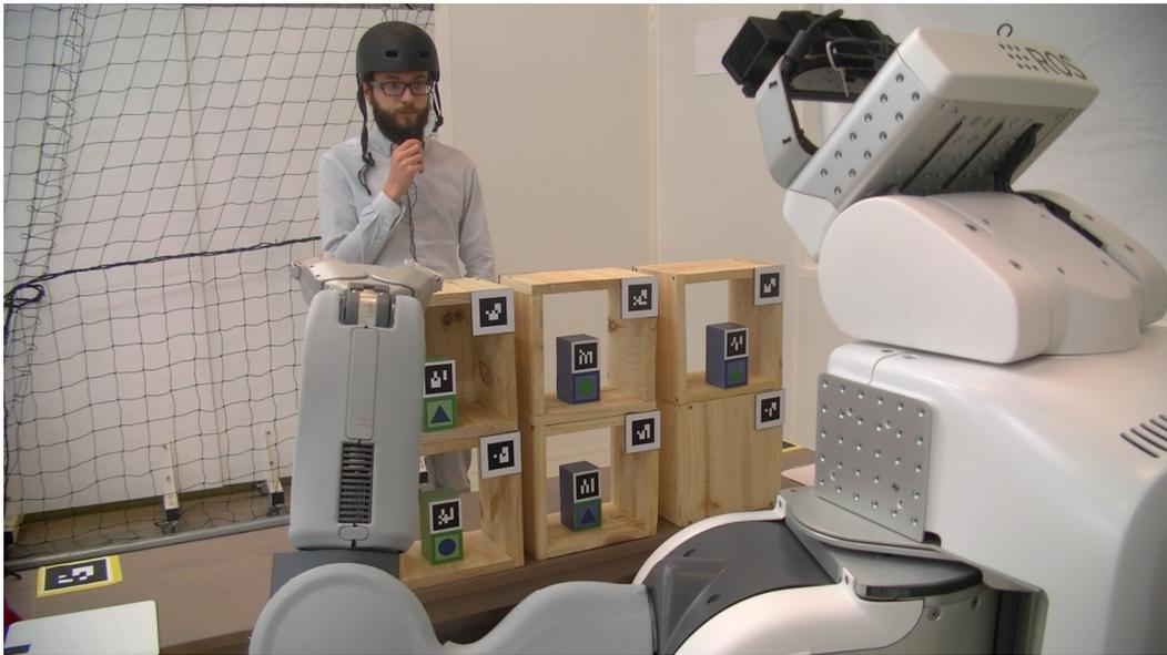
Figure 9.6 – Initial set-up of our Director Task demonstration from the robot perspective. One block is hidden from the human and one is hidden from the robot.
