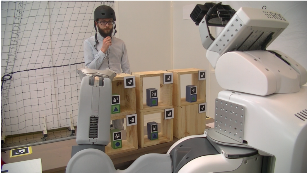
Figure 9.6 – Initial set-up of our Director Task demonstration from the robot perspective. One block is hidden from the human and one is hidden from the robot.
