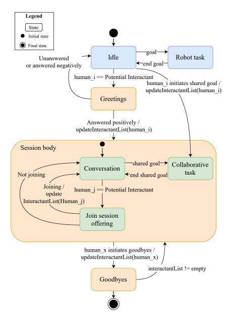
Figure 6.9 – States of the Interaction Session Manager (ISM). In blue are represented the states of the ISM when the robot is not in an interaction session. In orange are the states in which the ISM can be during an interaction session. In green are the sub-states of the interaction session body.
