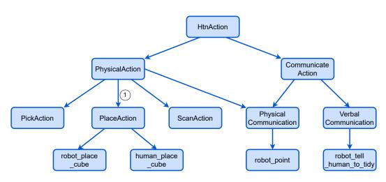
Figure 6.3 – The representation of an extract of the ontology class hierarchy graph of HTN actions. Taking the class PhysicalAction, the arrow ① has to be read as "A PlaceAction is a kind of PhysicalAction".
