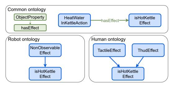
Figure 6.5 – Illustration of the human and the robot having differing ontologies. Both have the common knowledge that HeatWaterInKettleAction has isHotKettleEffect as effect. However, in the robot ontology, isHotKettleEffect is defined as a NonObservableEffect whereas in the estimated human ontology it is defined as a TactileEffect and a ThudEffect which are both ObservableEffect as shown in Figure 6.4.
