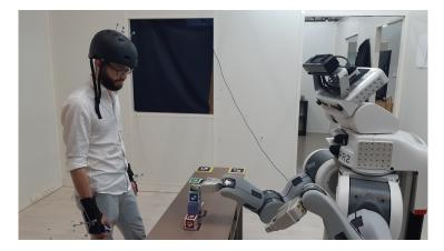
Figure 6.2 – The StackBuildingTask being performed by a human and a PR2 robot. The human is perceived through motion capture and the cubes with the Kinect on the robot head.
