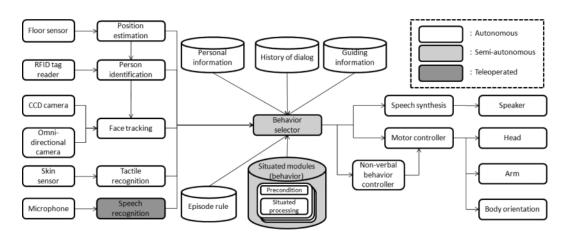
Figure 8.1 – Robovie system overview presented in (Kanda et al., 2010).
