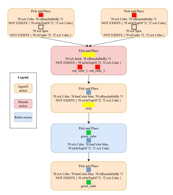
Figure 6.16 – A shared plan for the StackBuildingTask computed by HATP with modifications to generate SPARQL queries instead of object names as action parameters.
