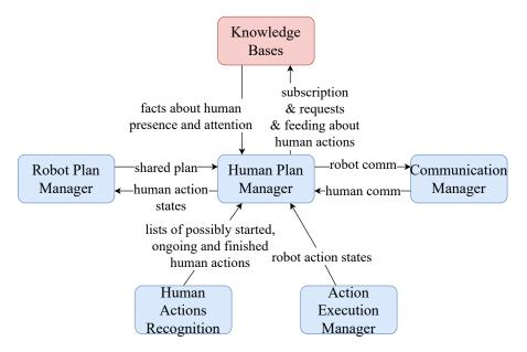
Figure 6.19 – The Human Plan Manager and the RJAs (in blue) and the component of the robotic architecture (in red) with which it interacts.
