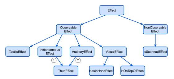
Figure 6.4 – The representation of an extract of the ontology class hierarchy graph of action effects. Taking the class ThudEffect, the arrows ① and ② indicate that ThudEffect is and an InstantaneousEffect and an AuditoryEffect.
