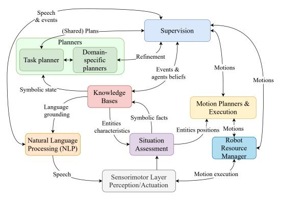
Figure 3.1 – Overview of the Deliberative Architecture for COllaborative roBOT (DACOBOT).
