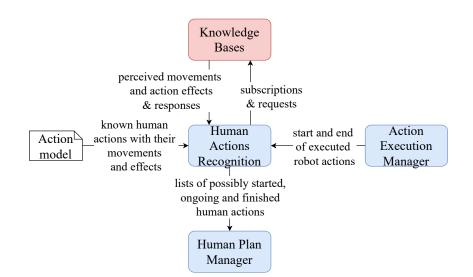
Figure 6.10 – The Human Actions Recognition and the RJAs (in blue) and the component of the robotic architecture (in red) with which it interacts. It is fed by a file (in white) with description of the human actions the robot should recognize.
