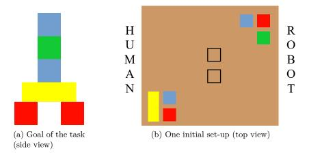
Figure 6.1 - Description of the blocks building task. The human and the robot have to build the stack together. We assume that the robot and the human know where all the available blocks are. We would like the robot to adapt as much as possible to the human actions and decisions while avoiding useless or tiresome verbal interactions.
