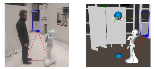
(b) The robot and the human are in their final positions. The blue spheres are the computed position for the human by the robot. The robot is pointing to the passage (in blue frame). We can observe the triangle formed between the human, the robot and the passage (the blue area on the floor) as in Figure 8.2 where two humans are in a triangle formation.
