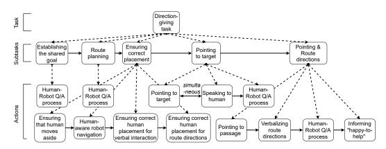
Figure 8.3 – The representation of the direction-giving task as a hierarchical task network with task, subtasks and actions levels. All the horizontal arrows are sequential links and the rest are decomposition ones.
