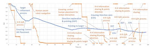
(c) Evolution over time of the measured QoI for the non-compliant human. Several times the human did not give the expected answer to the robot during the target refinement process. Then, they blocked the robot path. After that, the robot had to ask twice the human to come in front of it. Finally, the robot repeated the route direction three times but still the human kept saying that they did not understand. Therefore, the task QoI decreases all along the task.
