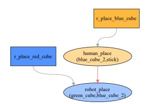
Figure 6.7 – An excerpt of the StackBuildingTask plan. The ellipses correspond to primitive tasks while rectangles represent abstract ones. The blue shapes are robot tasks and the yellow ones are the human ones. Finally, red arrows indicate the sequence of actions in the plans and gray ones represent hierarchical links, *i.e.* the links between the tasks as defined in the HTNs.
