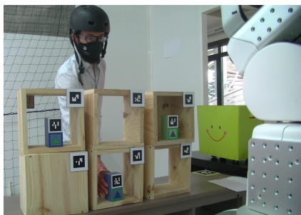
(e) The robot said “can you put the block with the blue triangle in the green storage box?”, thus the human is taking it. The other block with a blue triangle is not visible by the human.
