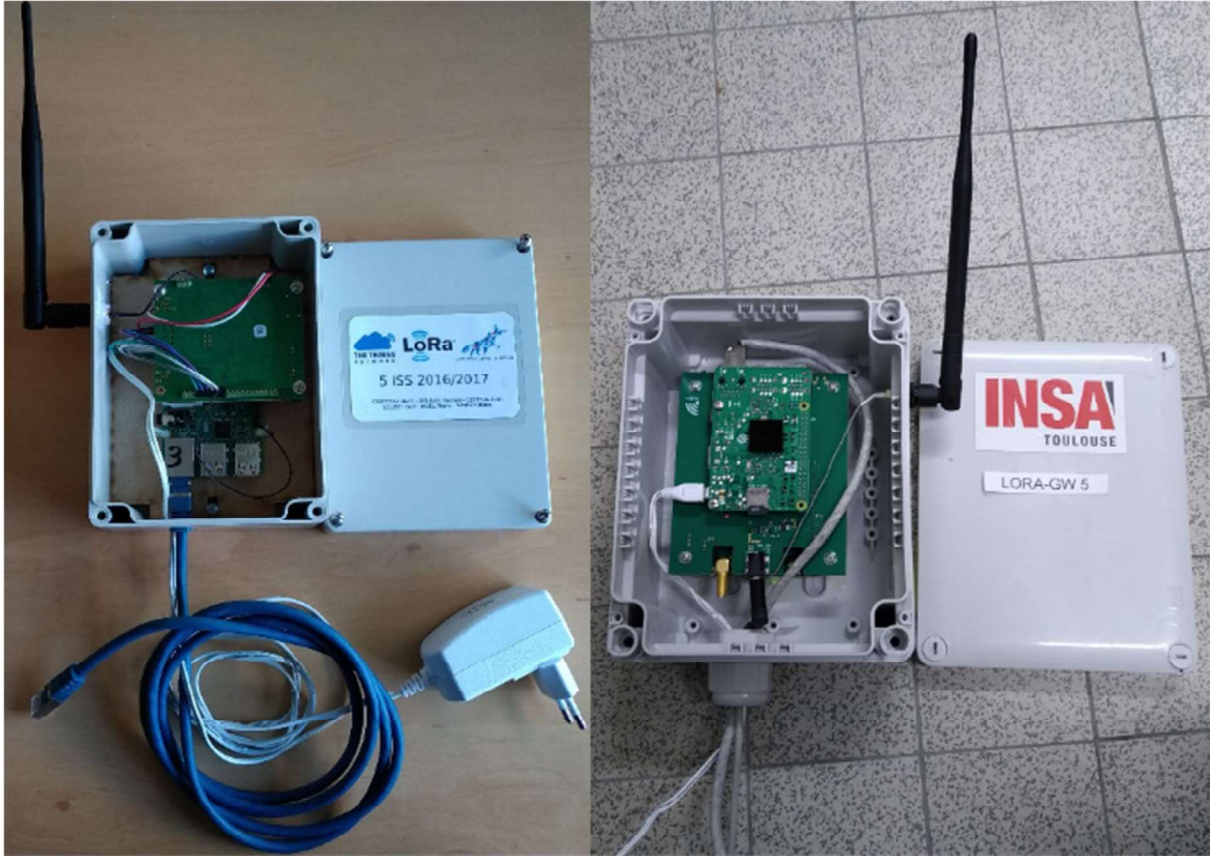
Figure IV.4: Photographs of the designed and implemented LoRaWAN gateways.
