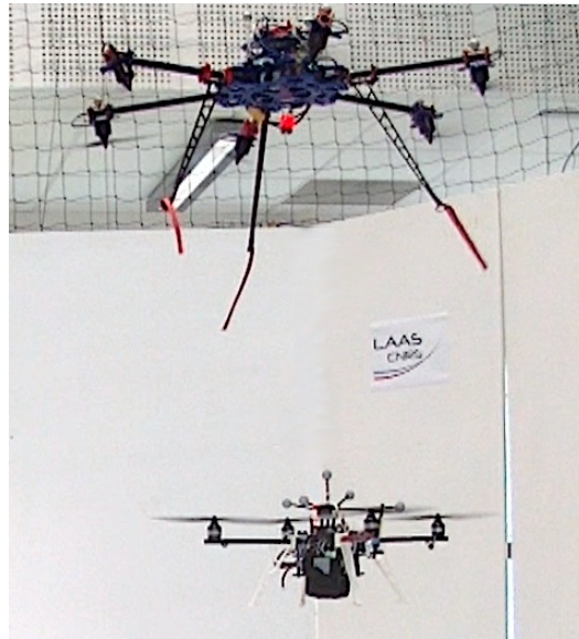
Figure 8.6 – The quadrotor flying stably beneath a 2.5 [Kg] hexarotor.
