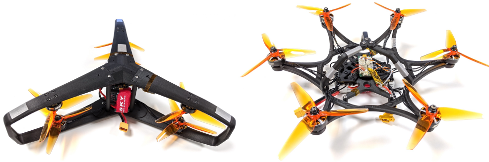
Figure 4.7 – The Y-shaped (left) and Star-shaped (right) hexarotor platforms built in-house for the fair comparison.
