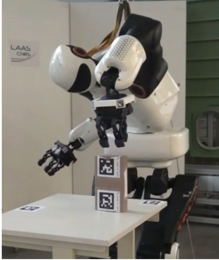
Figure 5.2: TALOS robot with AprilTag markers on its wrists
