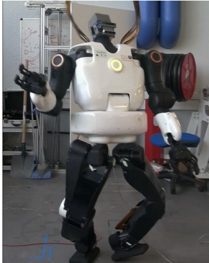
Figure 4.21: Failed experiment using torque control for a postural task.
