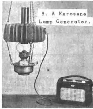
A KEROSENE LAMP GENERATOR.
