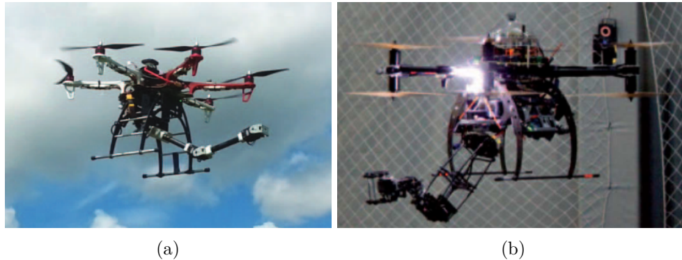
Figure 1.3: Second generation of aerial manipulators: (a) Flying Mobile Manipulator Unmanned Aerial Vehicle [Morton 2016]; (b) Aerial manipulator in an indoor environment [Muscio 2018]
