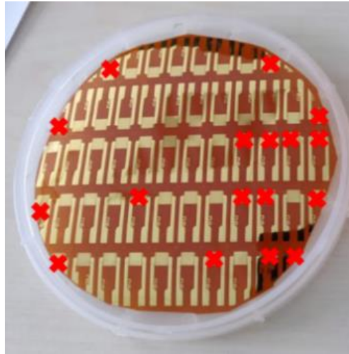
Figure 2.37 : Output of a 4-inch wafer with proper 3 \mu\text{m} gap separation between IDE is never 100%.
