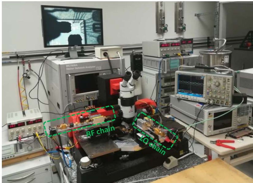
Figure 2-29: 60-90 GHz RF-probe measurement bench.
