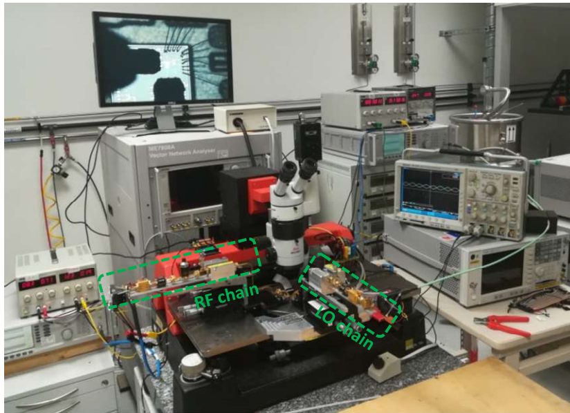
Figure 2-29: 60-90 GHz RF-probe measurement bench.
