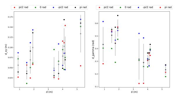
Figure 1.17: Linear distance (on the left) and local angular distance (on the right) between the average human trajectories and the generated trajectories according to the global distance for all orientations (in grey mean  $\pm$  standard deviation).
