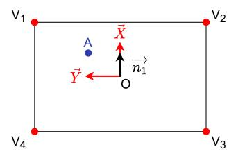
Figure 3.4: Robot support polygon representation.
