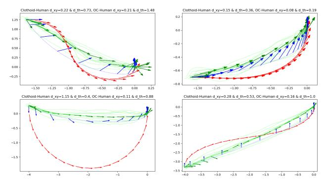
Figure 1.12: Examples of comparison between the 2 presented models (clothoid in red and OC in blue) and measurements on 10 subjects (average trajectory in  $bold\ green$  and measured trajectories in  $light\ green$ ) for starts 7, 8, 9 and 10.
