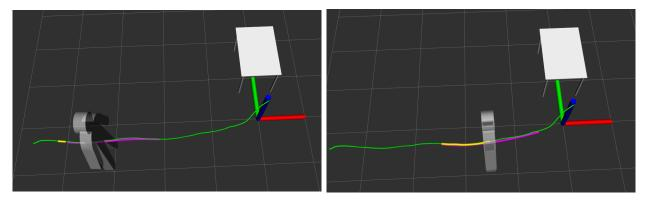
Figure 2.2: Example of the current predicted trajectory (in *purple*) of a human trajectory (in *green*) from his latest past trajectory (in *yellow*) with  $N_0 = 50$  and  $N_{OC} = 100$ .
