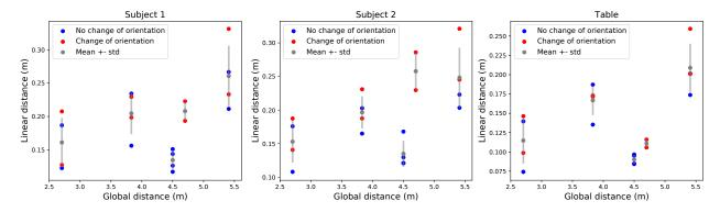
Figure 4.13: Mean linear distances between the average trajectories and the measured trajectories according to the global distance. In *blue* are plotted the distances for the trajectories which require a change of the table's orientation (Goal 2, 4, 6, 8) while the others are plotted in *red*. Let us denote, that there is an even number of points of each color for every global distances because there are two achievable configurations per goals.
