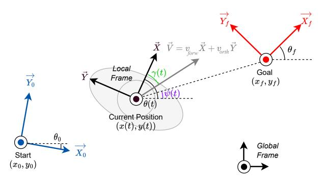
Figure 1.9: Representation of the coordinate systems and variables at stake in the OC problem to solve.
