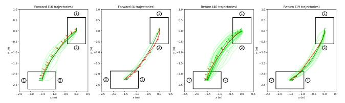
Figure 5.13: Comparison between table trajectories (average in *bold green* and measurements in *lime green*) and generated trajectories (in *red*) for one goal position (Goal 8 on Fig.5.12). The arrows represent the orientation of the table during locomotion and the number 1 and 2 the position of both subjects at the beginning and at the end of the motion.
