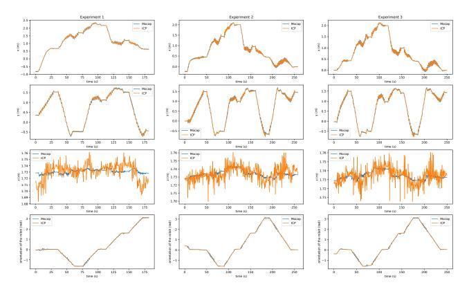
Figure 5.11: Position (x on the first row, y on the second row, z on the third row) and orientation ( $\theta$  on the last row) of the robot measured by the MoCap (in blue) and by the ICP localization system with the removed delays and structural offsets (in orange) during the 3 experiments
