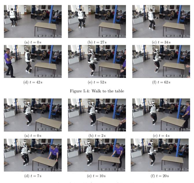
Figure 5.5: Tracking of the table (Translation of the table toward the robot at t = 2 s and rotation of the table at t = 10 s)
