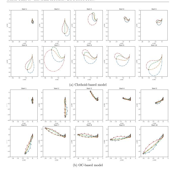
Figure 1.11: Generation of all the trajectories with the same starting and goal positions than during the experiments. The goal position always is  $(x_f, y_f) = (0, 0)$  with  $\theta_f = \frac{\pi}{2}$  rad. On each plot, there is one trajectory per starting orientation  $(\theta_0 = -\frac{\pi}{2}$  rad in *blue*,  $\theta_0 = 0$  rad in *orange*,  $\theta_0 = \frac{\pi}{2}$  rad in *green* and  $\theta_0 = \pi$  rad in *red*).
