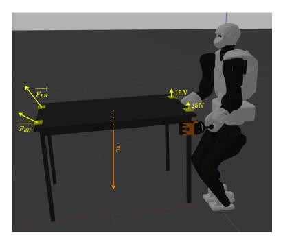
Figure 5.20: Simulation on Gazebo where a TALOS humanoid robot holds a 20.7 kg table.  $\vec{P}$  is the weight of the table.  $\vec{F}_{RH}$  and  $\vec{F}_{LH}$  are the forces applied on the left yellow spots to simulate the forces applied on the table by the hands of the human partner.
