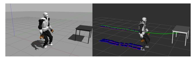
Figure 3.9: Simulation on Gazebo (*left*) of the robot executing the predicted trajectory with  $N_0 = 50$  and  $N_{OC} = 100$ . The CoM, footsteps (desired in *red*, real in *blue*) and human trajectories (in *green*) are also displayed in RViz (*right*) for comparison.
