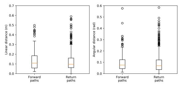
Figure 5.14: Linear and angular distances between the individual table trajectories and the average trajectories for every goal.
