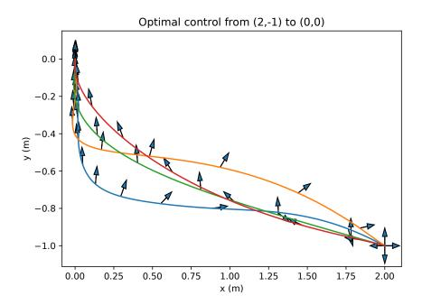
Figure 1.10: Trajectories from  $(2, -1, -\frac{\pi}{2})$ , (2, -1, 0),  $(2, -1, \frac{\pi}{2})$  and  $(2, -1, \pi)$  to  $(0, 0, \frac{\pi}{2})$  generated with an OC model adapted from Mombaur et al. [38] (respectively in blue, orange, green and red). The arrows represent the current orientation of the system during the gait.
