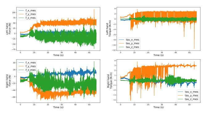
Figure 5.22: Forces and torques measured during the simulation by the 6-axis force sensors placed on the right and left hands.
