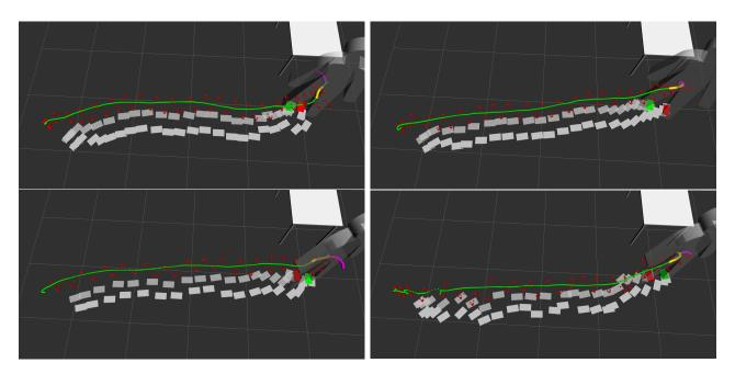
Figure 3.11: Result of the coupling of the prediction model and the WPG for 4 different human subjects. The CoM trajectory of the human is in *green*, the CoM trajectory of the robot is in *red* and the performed footsteps of the robot are in *grey*.
