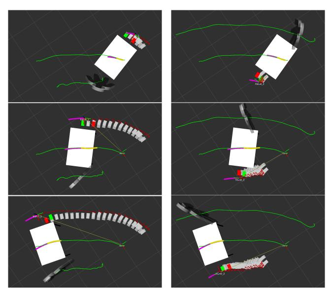
Figure 5.17: The robot CoM (in red) and footsteps (past steps in grey, current support foot in red and future support foot in green) are generated from the predicted table trajectory (in purple) with  $N_0 = 50$  and  $N_{OC} = 100$ . On the left, the robot substitutes Subject 1 while, on the right, it substitutes Subject 2.
