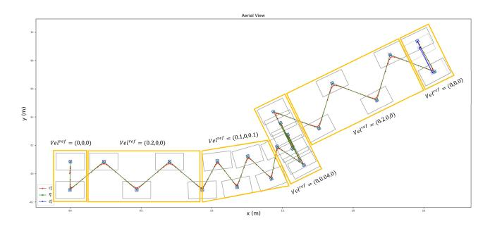
Figure 3.5: Generation of CoM and footsteps trajectories with the WPG with velocity tracking.
