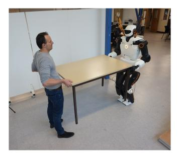
Figure 2: Human-robot collaborative load-carriage task.
