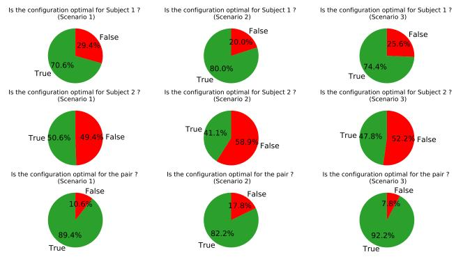
Figure 4.10: When the table configuration minimizes the traveled distance of Subject 1, Subject 2 and the pair, it is called optimal. These pie charts show the percentage of experiments where the pair put the table in an optimal configuration for Subject 1 (at the top), for Subject 2 (in the middle) and for the pair (at the bottom) according to the different scenarios.
