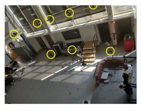
Figure 5.2: Experiment room (the Qualisys cameras are circled in yellow).
