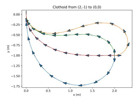
Figure 1.8: Clothoids from  $(2, -1, -\frac{\pi}{2})$ , (2, -1, 0),  $(2, -1, \frac{\pi}{2})$  and  $(2, -1, \pi)$  to  $(0, 0, \frac{\pi}{2})$  generated with a fitting algorithm (respectively in blue, orange, green and red).
