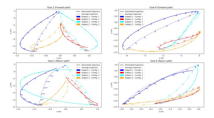
Figure 4.16: Average (dotted line) and generated trajectories (full line) for both subjects, with both configurations when measured. The arrows represent the orientation of the pelvis of the subjects during locomotion.
