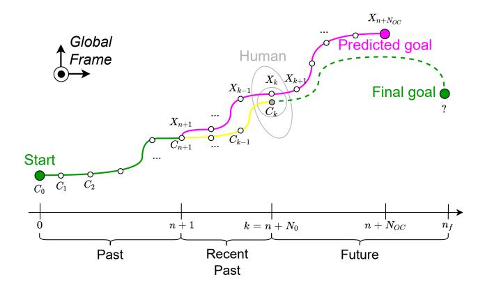
Figure 2.1: Prediction problem representation at time  $t = kT_{OC}$  with  $k = n + N_0$  (in green and yellow the whole past human trajectory, in stippled green the unknown future human trajectory and in purple the predicted trajectory).
