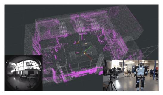
Figure 5.8: Frame extracted from the video of the first experiment. The video shows the ICP data (prior map in *grey*, read point cloud aligned in *pink*, axis: estimated pose) and the targeted poses (arrows) in the middle, the image from a sensor of the Intel RealSense T265 on the left and the video of the experimental room and the robot on the right.
