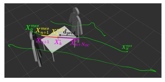
Figure 5.16: Predicted trajectory at time  $t = kT_{OC}$  with  $N_0 = 50$  and  $N_{OC} = 100$  for one given trial. The measured trajectories of both subjects and of the table are in *green*, the recent past trajectory of the table is in yellow and the solution provided by the prediction process is in purple.
