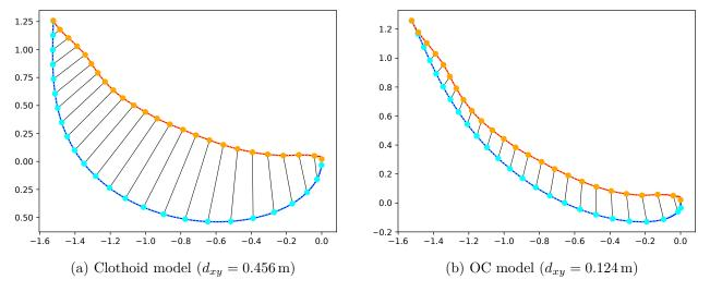
Figure 1.13: Linear distance between a measured (*blue*) and a generated (*orange*) trajectory with N=25.
