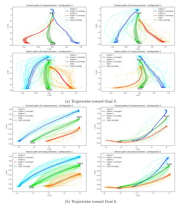
Figure 4.4: Trajectories performed by each pair and average trajectories during Scenario 3 for two different goals. The trajectories performed for these two goals are typical of the observed straight (Goal 2) and oblique (Goal 6) motions. The arrows represent the average orientation of the pelvis of Subject 1 (in blue) and Subject 2 (in red) and of the table (in green) during locomotion.
