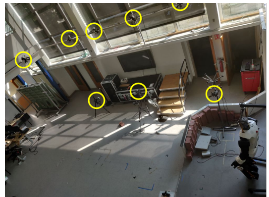
Figure 5.2: Experiment room (the Qualisys cameras are circled in yellow).
