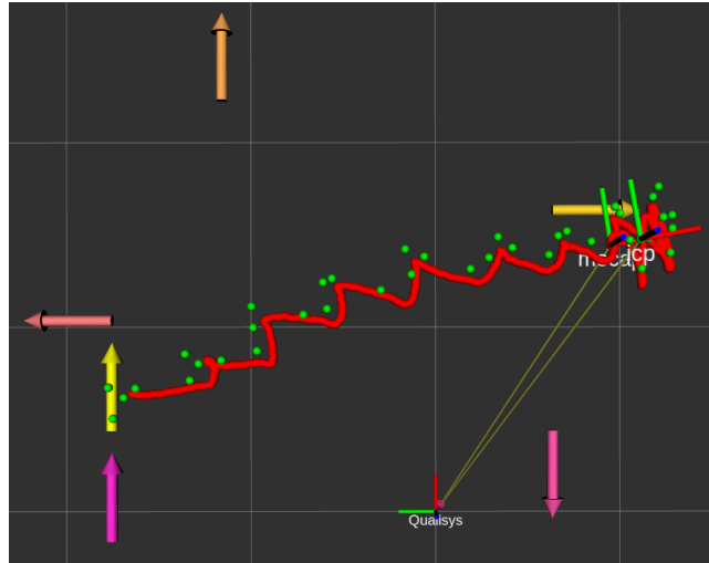
Figure 5.9: Visualization of the recorded data on Rviz (in red the MoCap set and in green the ICP set)
