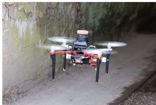
(b) A UAV entering the mine in the DARPA Subterranean Challenge (courtesy of [Rouček, 2019]).
