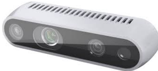
(b) The D435, a stereo infrared RGBD camera.
