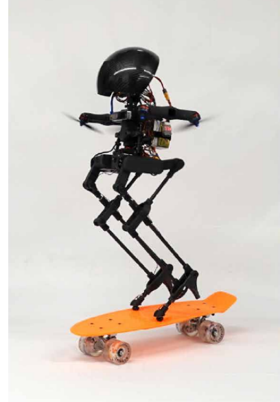
(b) LEONARDO: A bipedal robot equipped with two rotary wings (courtesy of [Kim, 2021]).
