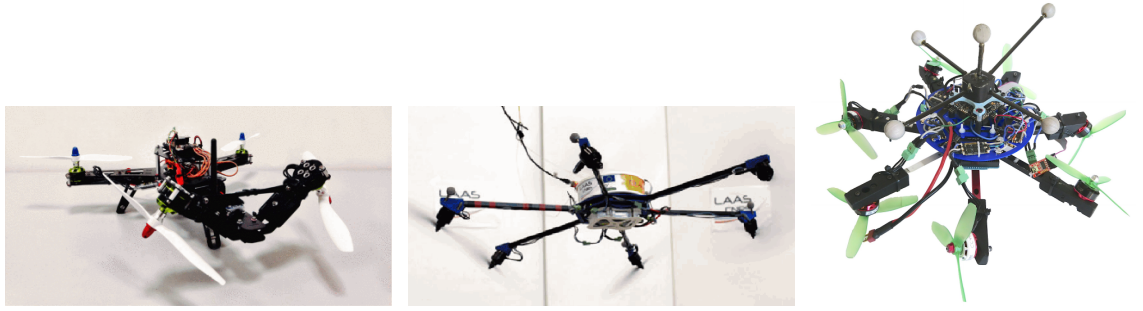
(a) A V-tail quadrotor, with two tilted propellers (courtesy of [Ciarfuglia, 2014]). (b) The Tilt-Hex, a tilted-propeller hexarotor developed in the LAAS-CNRS (courtesy of [Bicego, 2020]). (c) The Omni7+, an omnidirectional heptarotor (courtesy of [Hamandi, 2020]).
