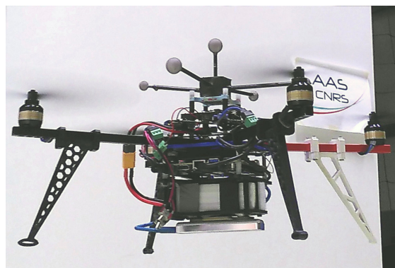
(b) Snapshot of a flying quadrotor with a down-facing camera, used the experiments from Chapters 6 and 8.
