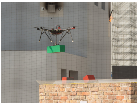
(a) A UAV performing a fully autonomous brick pick-and-place on a wall mock up, in the MBZIRC 2020 challenge (courtesy of [Lenz, 2020]).
