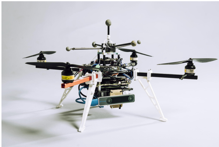
Figure A.1: Snapshot of a quadrotor used in the various experiments. It is equipped with MoCap reflecting balls on top and a front-facing camera.
