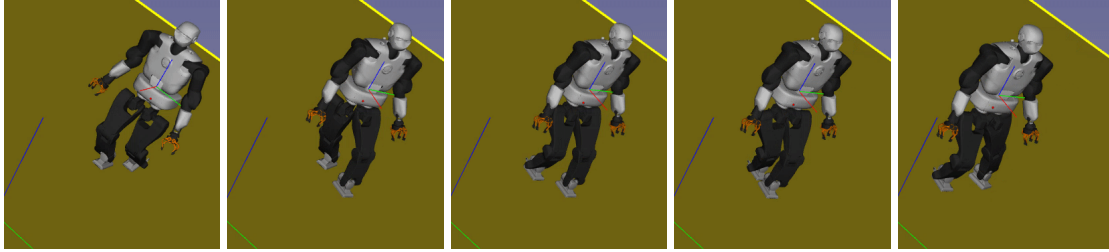
Figure 4.18: Without reward on the orientation, LEAS-P2 learns that the sidewalking strategy is the most robust and successful with SBCP.
