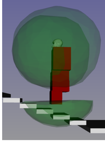
Figure 3.2: Validity constraints of the Talos Robot, (green) ranges of motion of each end effector, and (red) the robot trunk. The configuration above is valid as the robot can potentially reach the ground ( \mathcal{R} ) and the trunk is not in collision with the terrain ( \mathcal{C} ).
